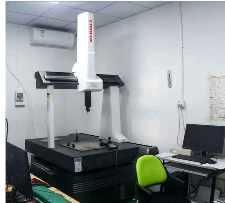
Hexagon Croma CMM machine . Measure range 1000*800*600mm
