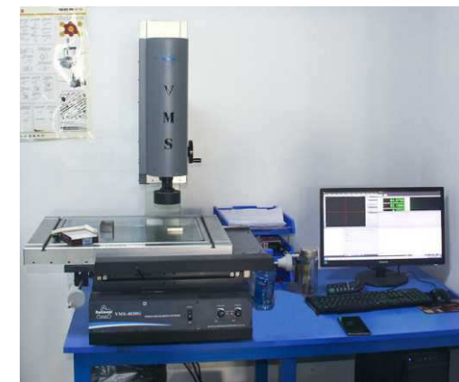
VMS Projector, measure capacity 400*300*200
